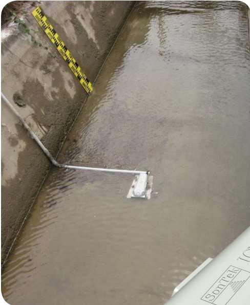
SonTek-IQ canal installation as part of a HydroMet station
