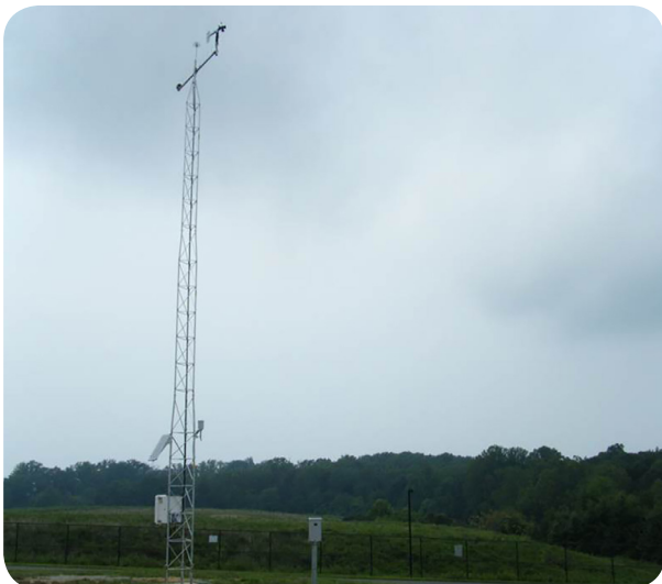
Monitoring tower containing a YSI Data Logger and meteorological sensors
