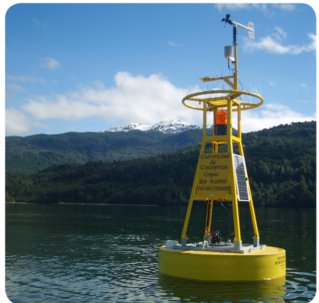
Monitoring Buoy containing meteorological sensors.
