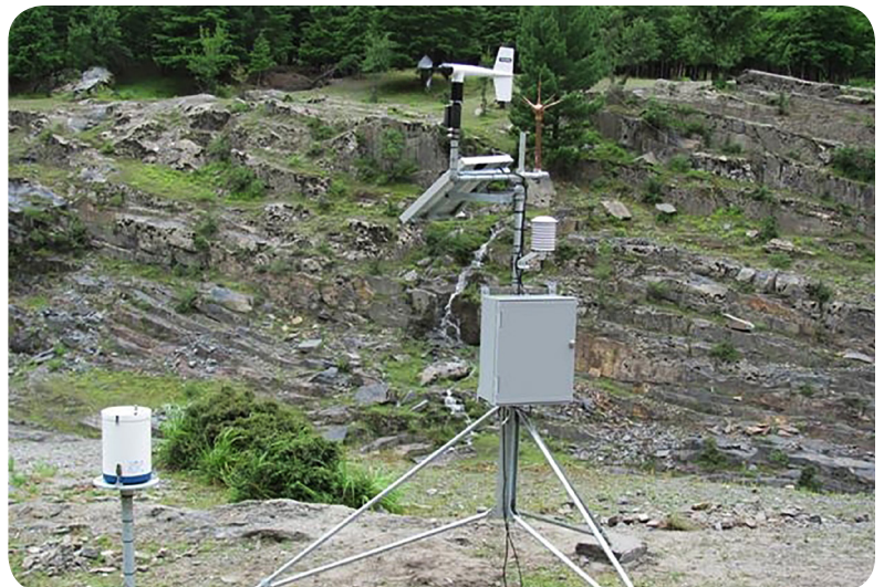
Turn-Key monitoring station containing a YSI Data Logger, Rain Gauge and other meteorological sensors.
