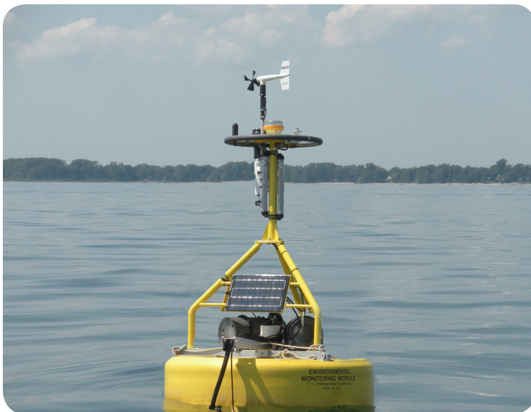
Monitoring Buoy containing meteorological sensors.
